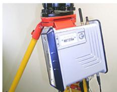
In land surveying applications, when used as a roaming base mounted on a tripod, the ProFlex 800 can be secured on one of the legs of the tripod using the lug located on its bottom side.
