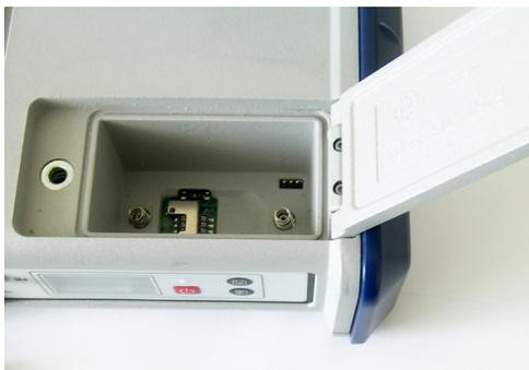
The battery used is a 7.4-V DC - 4600 mAh rechargeable battery. It is a standard model used in many camcorders. The battery is housed in a battery compartment accessible from above the ProFlex 800. The compartment door can be opened by lifting and then turning the quarter-turn finger screw counter-clockwise.
