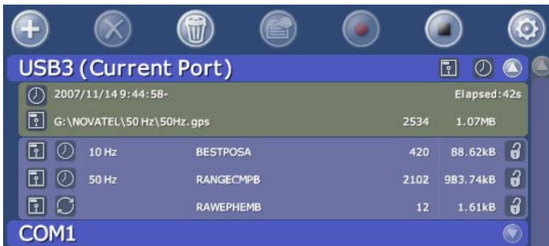
Figure 13: 50 Hz Logging Example in CDU
