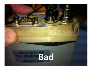
When you are reinstalling the end cap screws be sure that the gaskets are not exposed between the connection. Once the screws are back in the end caps, you can put the mounting bracket and rubber end guards back on.
