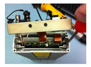
After the battery has been unplugged remove the 2 battery retaining bracket screws.
