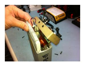
When the bracket has been removed go to the other side of the receiver and open the end cap. You will need to push the battery from that end toward the back, it is a fairly tight fit. When the battery is exposed enough through the back of the receiver you can pull it the rest of the way out.
