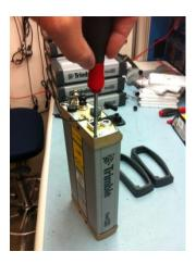
Next, using your torx screw driver remove the 4 screws holding on both the front and back end caps.
