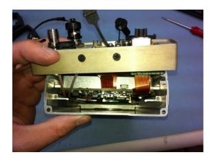
To reinstall the battery you will only need to remove the back end cap of the receiver (see instructions above for that process). Once the end cap is removed you will need to remove the battery retaining bracket which will expose the empty slot where you will slide the battery into.
