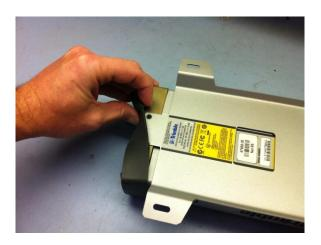
If the mounting bracket is still attached, remove the rubber end guards to expose the connection screws. Remove the screws on both ends.
