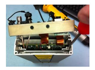
Before you slide the battery back in, ensure that the side with the wires coming out is on top. After the battery is inserted reinstall the retaining bracket and plug the connector back into the terminal. You will then once again put the end cap back onto the receiver body (see instruction above) ensuring proper alignment of the sealing gasket.
