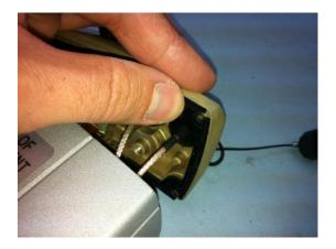
When the battery is out, be sure to reinsert the battery retaining bracket into the receiver with the 2 screws. Now you are ready to reattach the end caps of the receiver. Be sure that the rubber gaskets are properly seated in their grooves as you are fitting them back on the receiver.
